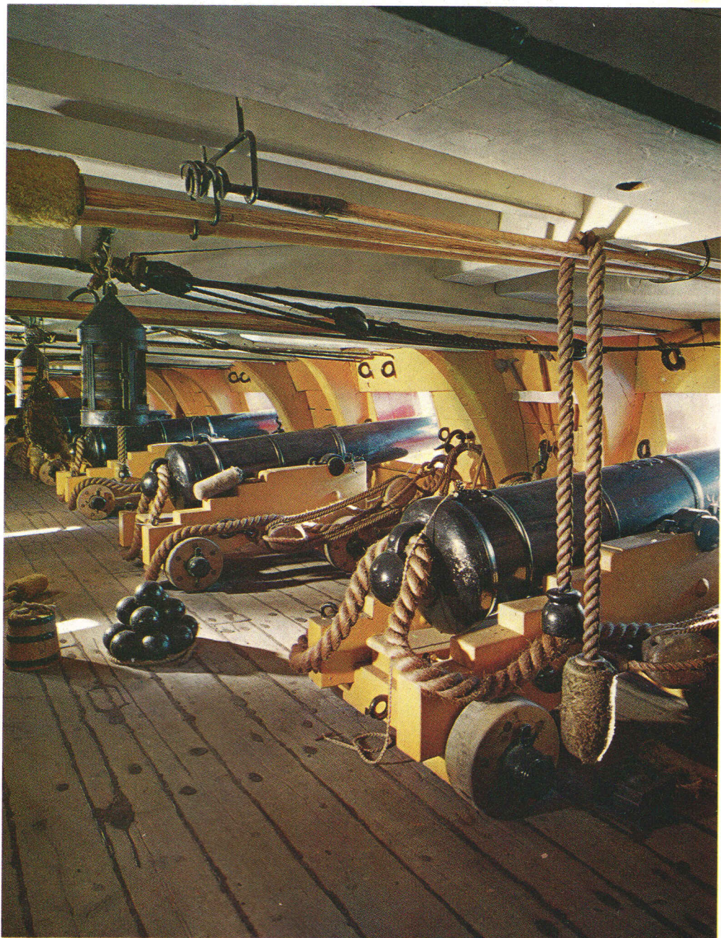
Gun-decks were festooned with gear: shot was stacked on the deck and flexible rammers snaked down from deckheads where the gunners' tools were racked in neat rows.
