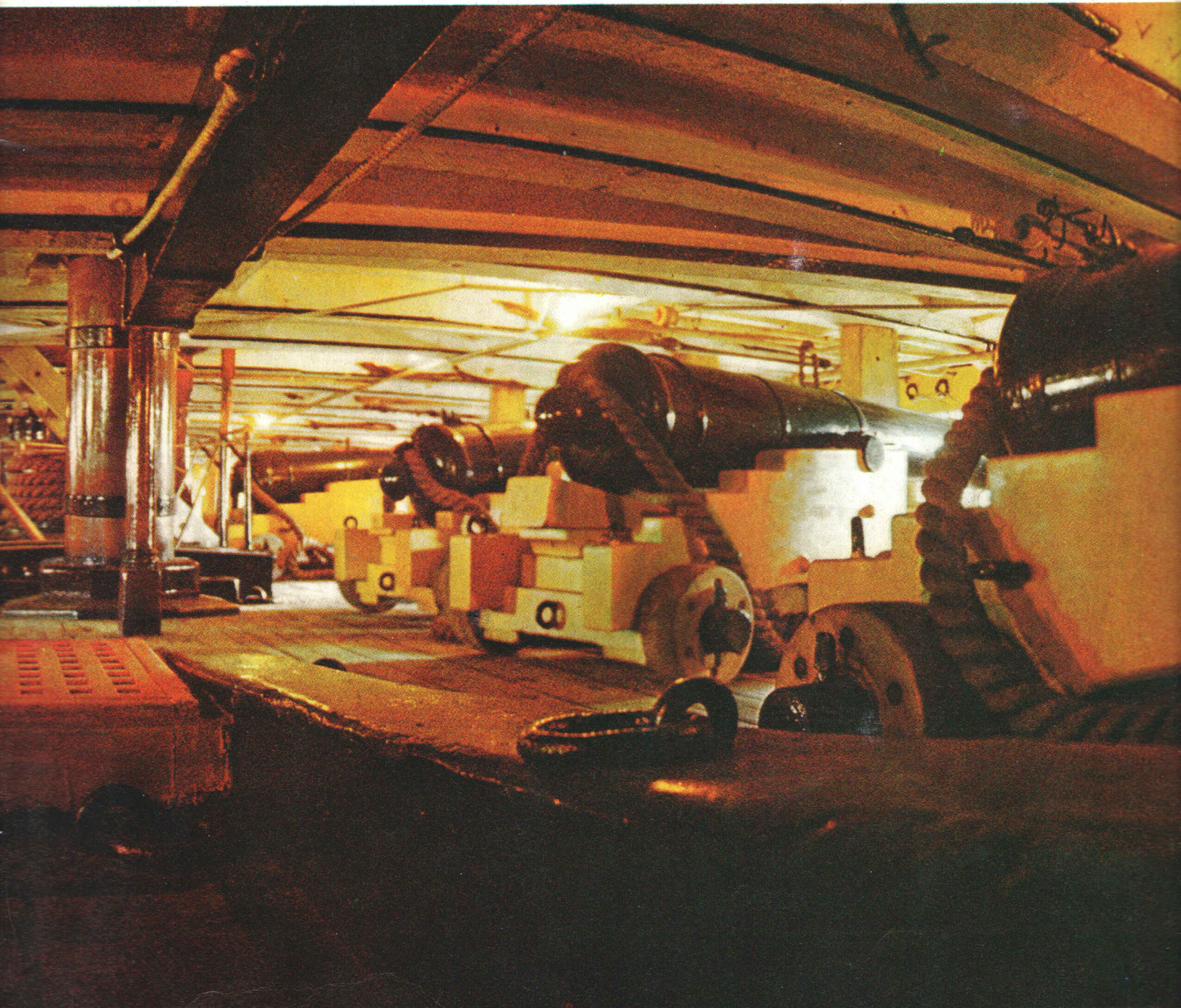
They recoiled violently after each firing. A 15-man crew was needed to serve each pair of port and starboard guns.
